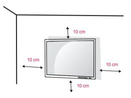
To install the monitor to a wall, attach a wall mounting bracket (optional) to the back of the monitor. Make sure that the wall mounting bracket is securely fixed to the monitor and to the wall.
